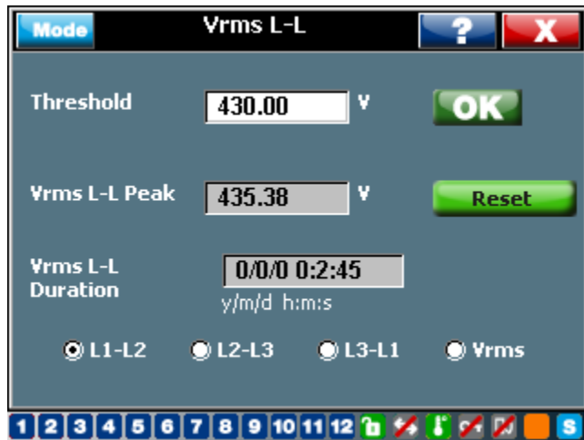
Figure 24: Event logging threshold setting - Vrms
