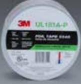
High Strength foil tape printed with UL listed label. Specifically designed for use fiberglass duct board systems. Use with rigid glass fiber air duct board (181A-P) and flexible (non-metallic) air ducts and air connectors (181B-FX). UL® Listed meets requirements of UL 181A-P and UL 181 B-FX                                      | 4.0 mil   | 121°C<br>250°F       | 2.5" x 50 yd (63 mm x 45,7 m)                                                                      |
